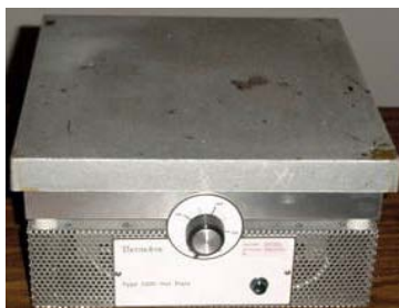
Thermolyne Type-2200 Hot Plate, Model HPA2235MQ 120V, 13.3A, 1600W, 50/60Hz, Phase-1 (7 available)
